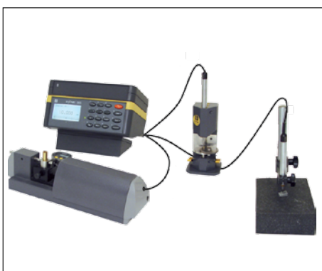
Using 3 measuring channels with 3 separated probes
