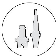
XL length toolholders are standard in the REGO-FIX product range and are immediately available. Their long and slim design allows for precise machining even with limited space.
