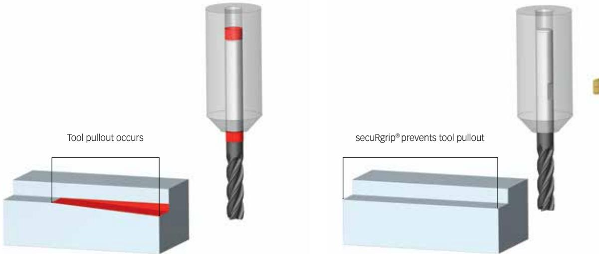
Length alterations can lead to damage of the workpiece.
