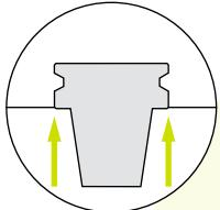
Higher colletholder stiffness due to taper (AT1) and face contact.
