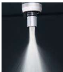
Tool periphery Coolant is supplied through slits of the tap holder.
