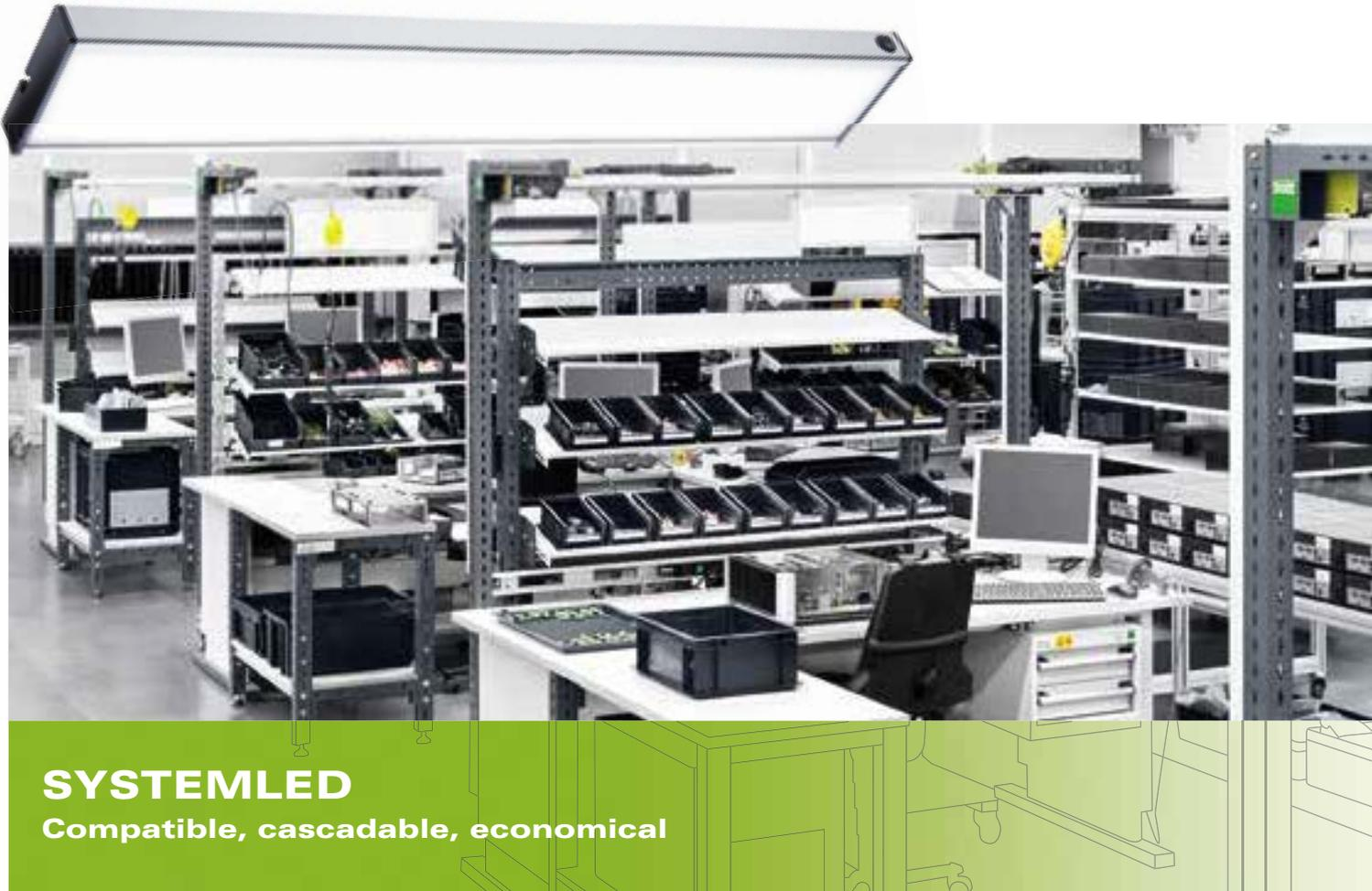
Developed for system workstations, the SYSTEMLED enables absolutely fast and simple replacement of fluorescent tube luminaires with LED luminaires. This is why the SYSTEMLED has the same dimensions and connections as the leading conventional luminaires. The electrical interlinkability of the SYSTEMLED makes it possible to create large, particularly efficient lighting surfaces.
