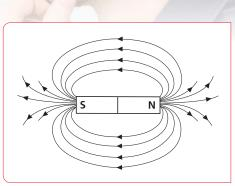
Single pole operation magnet flux crosses a gap but has a diminishing strength field.
