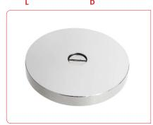
To achieve the optimum pull force, 100% contact area must be achieved using the recommended armature plate. The force will be affected if other material specifications, thickness and surfaces are used, or if the armature fails to make positive contact over the full diameter of the face of the magnet. Where misalignment is likely to be an issue we recommend that an oversized armature plate is used to ensure 100% full contact, this however will reduce the stated pull force by approximately 10%
