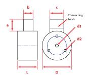
40, 50, 65, 80, 100mm diameter. 12VDC & 24VDC. Two pole connector
